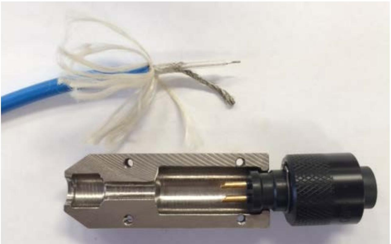
E. The wire lengths should be about 1 inch when finished trimming.
