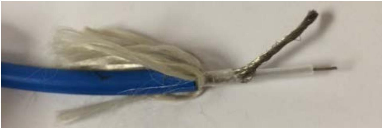
F. Slide a ½ inch piece of water tight shrink tube over the center conductor before soldering. It is not necessary to use water tight shrink tube on the shield. Use a small piece of 1/8 inch shrink tube to keep the shield from spreading and leave enough room exposed to slide into the connector.
