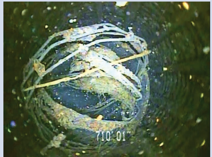
Downhole video camera view of loose wire in a well. Photo courtesy Eric Hadden, Laval Underground Surveys in Fresno, California.
