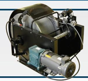
Driven by variable speed, high torque hydraulic (or optional electric) motor with 4,000 feet (1,219.2 m) of cable length. Features hand operated brake with eight square inches braking surface, and a dog clutch which allows winch drum to free spin.
