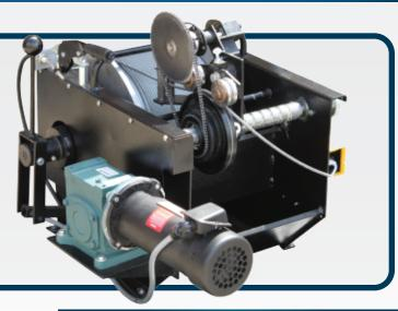
Driven by variable speed, high torque hydraulic (or optional electric) motor with 2,500 feet (762 m) of cable length. Features hand operated brake with 8 sq. inches braking surface, and a dog clutch, which allows winch drum to free spin.
